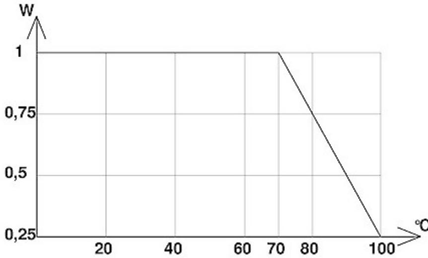
**Derating curve:** Potentiometers are derated from 100% rated dissipation at 40°C to 25% rated dissipation at 70°C.
